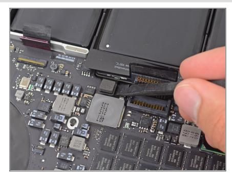
Use the flat end of a spudger to pry the battery indicator connector up from its socket on the logic board.
